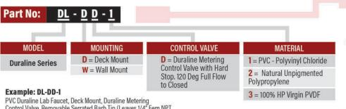
Control Valve, Removable Serrated Barb Tip (Leaves 1/4" Fem NPT Outlet when Removed), 3/8" Fem NPT Supply Inlet Connection
